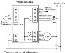
Two-pipe system with three-wire motorized valve (parameters need resetting)
