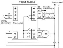
Four-pipe system with two-wire motorized valve
