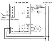
Two-pipe system with two-wire motorized valve
