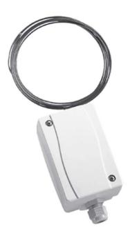
The frost protection thermostat STT is used for air, or water-side temperature monitoring of heat exchangers, hot water circulation systems, water / air heaters, e.g. in ventilation and air conditioning systems and for the prevention of frost damage. The product features a small operating differential and high reproducibility. Resetting of the STT900 to STT904 occurs automatically, and the STT910-STT914 are designed to be reset manually by a reset button.
