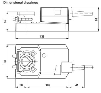
With utilisation of a round spindle made of CrNi (INOX): Ø 12...20 mm
