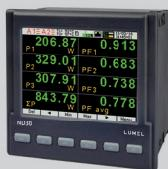
**ND30** - power network meter with Ethernet and recording
