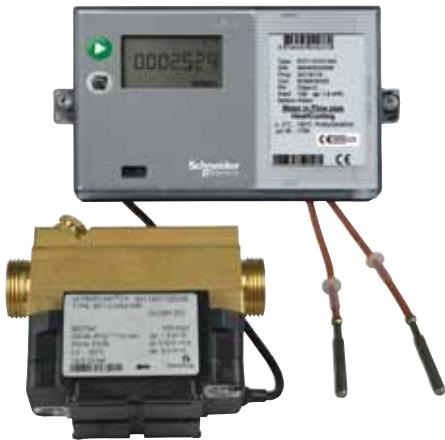
MULTICAL® 602 and ULTRAFLOW® 14/54 are used for measurement of cooling or combined heat/cooling in all water based plants with flow temperatures from 2°C to 50°C/ 90°C and with ULTRAFLOW® 14/54 between qp 1.5 m<sup>3</sup>/h and qp 400 m<sup>3</sup>/h.
