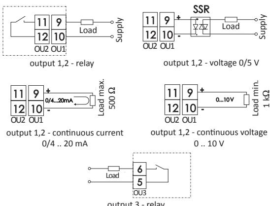
Fig. 2. Control/alarm outputs.
